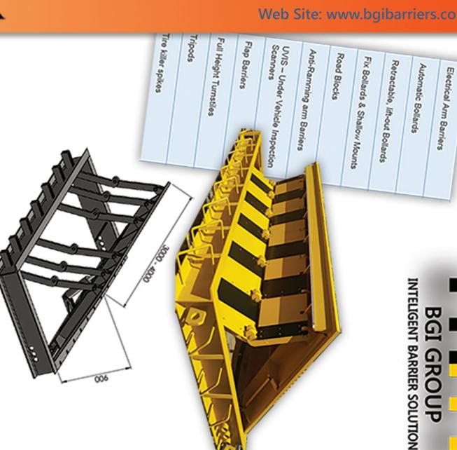
The R3000 is a shallow mounted ROAD BLOCK, high security K12 rated, able to stop a 7,500 kg truck moving at a speed of 80 kph. This product must be installed within an approved reinforced concrete foundation.
